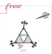
Parabole ILIAD Ø 0.70m HMA :43.30m AZ: 256\*
